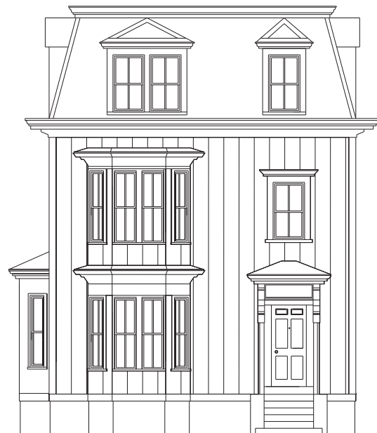
▲ Inappropriate Vertical siding.
