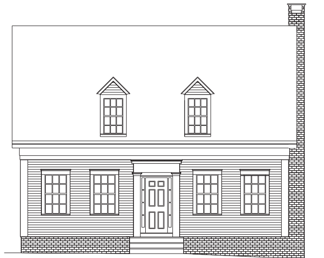
▲ Inappropriate Replace shingles with clapboards.
