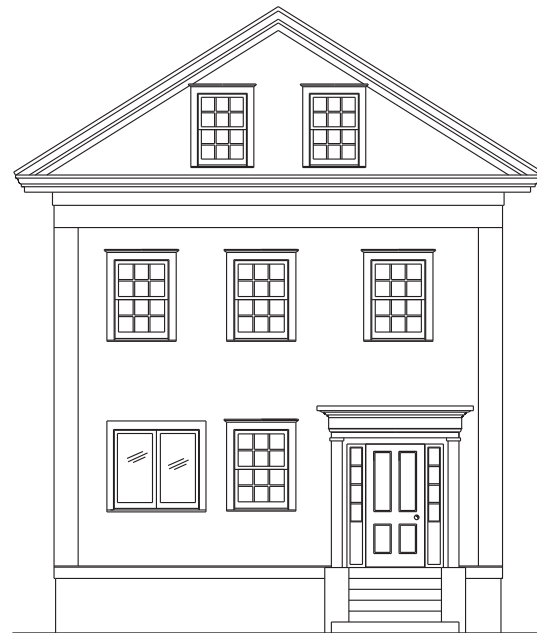
▲ Inappropriate Replacement single-pane casement window with enlarged opening. Missing drip caps.
