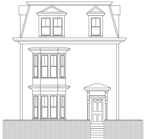
▲ Inappropriate Stockade fence exceeds height limits.
