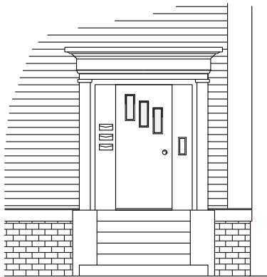
▲ Inappropriate Sidelights replaced by mailboxes and buzzers.
