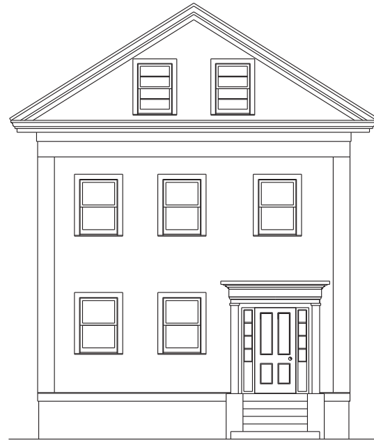
▲ Inappropriate Horizontally divided window replacements have incorrect number of panes. Missing drip caps.
