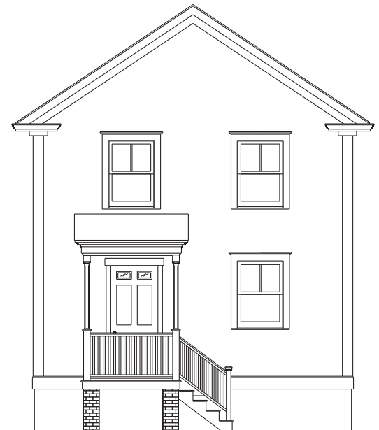
▲ Inappropriate Brick or wood columns without infill.
