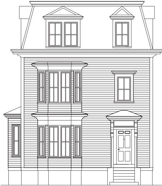
▲ Appropriate Original clapboards.
