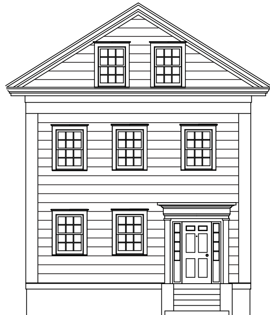
▲ Inappropriate Clapboards are too wide.
