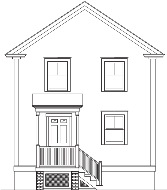
▲ Appropriate Brick or wood columns with infill.
