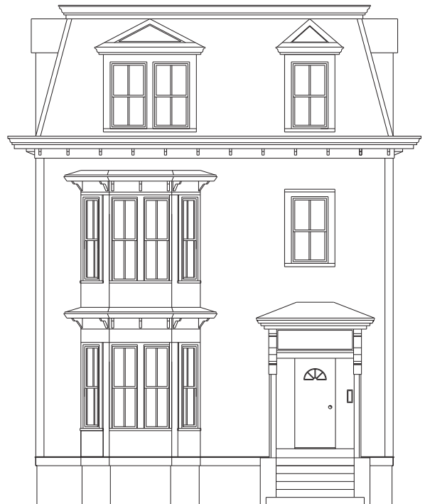
▲ Inappropriate Single door instead of double door. No panels. Non-historic glass panel design.
