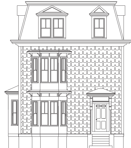
▲ Inappropriate Asphalt shingles, windows filled in.
