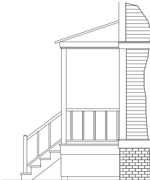
▲ Inappropriate Balusters are too far apart. No visual support for column. No cap on railing post. Lack of molding on roof. Lack of detail on column.
