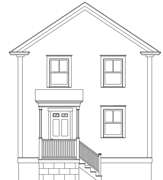
▲ Inappropriate Cinderblock porch base.
