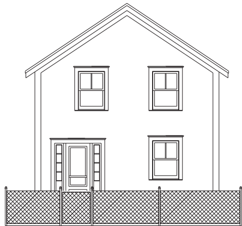
▲ Inappropriate Woven wire fence.
