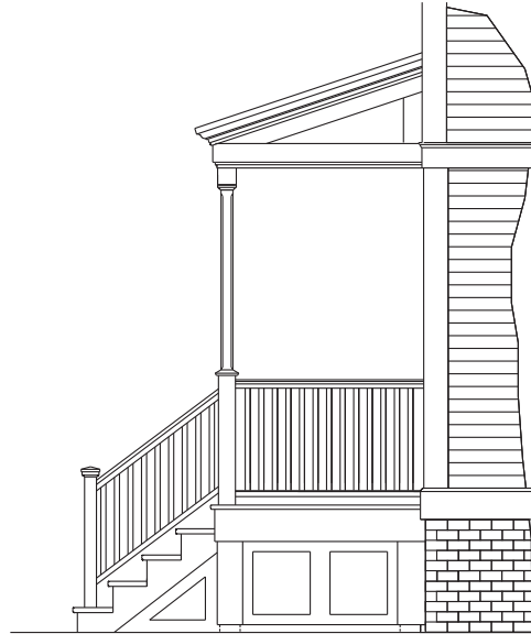
▲ Appropriate Balusters at appropriate distances; typically spaced at 4" on center. Cap on railing posts.
