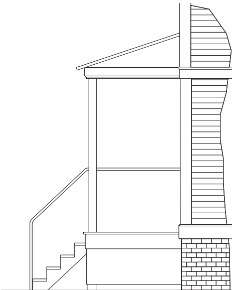
▲ Inappropriate Metal pipe railing. Lack of detailing on column and railing. No visual support for column. No stair nosing.
