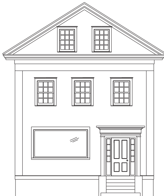
▲ Inappropriate Enlarged window opening for picture window. Window filled in.
