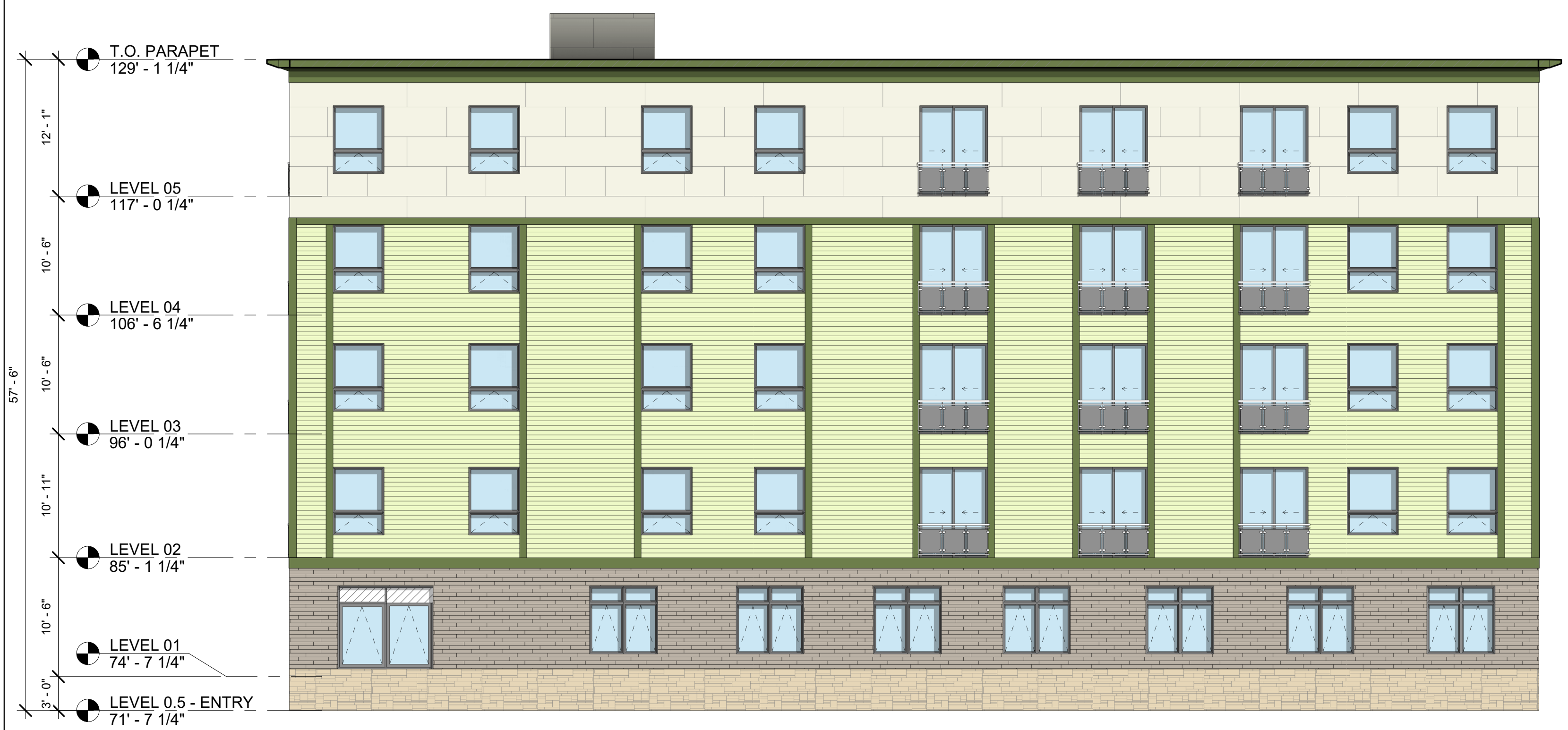
A-5 EXTERIOR ELEVATION - NORTH
