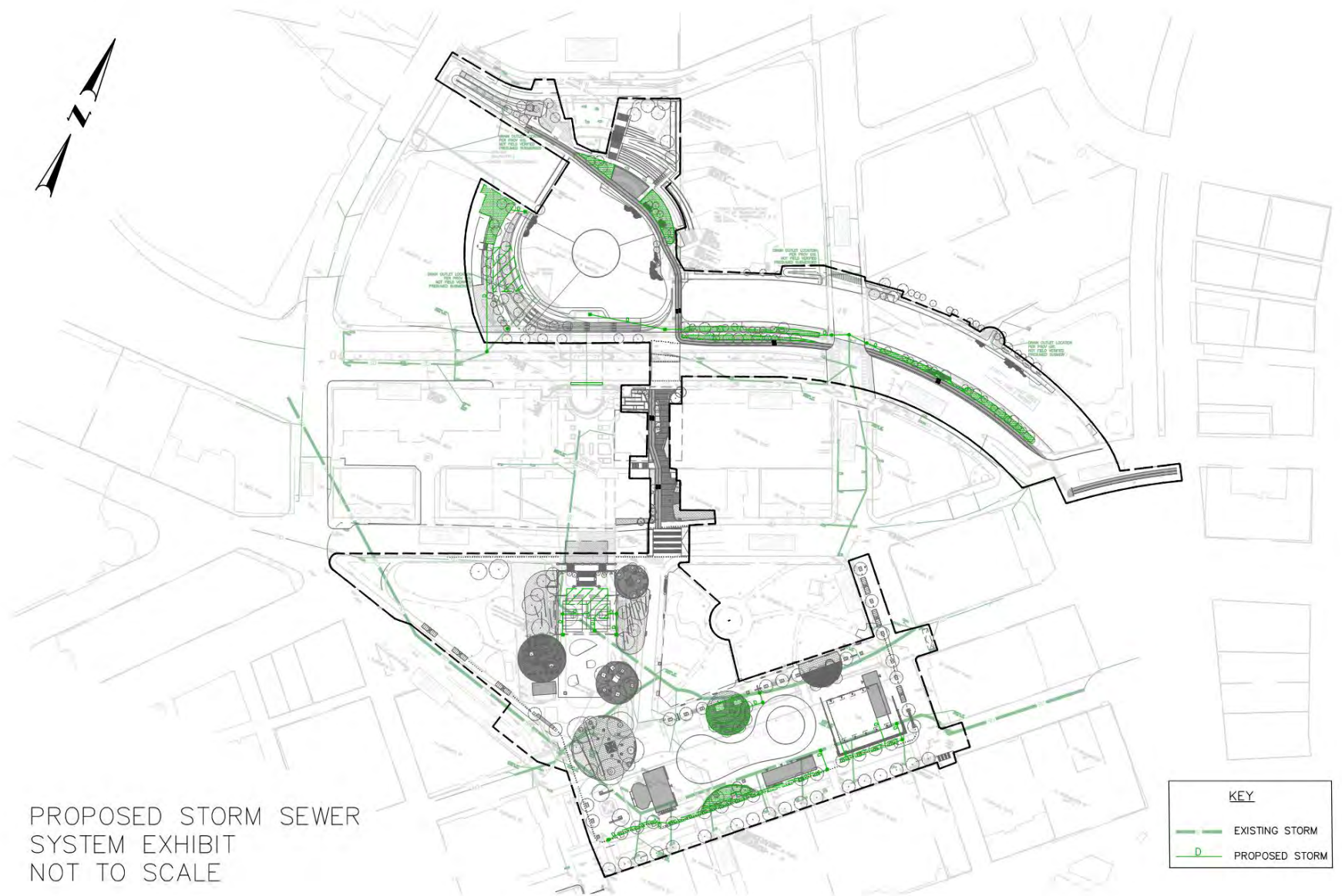
Figure 6 - Proposed Storm Sewer System
