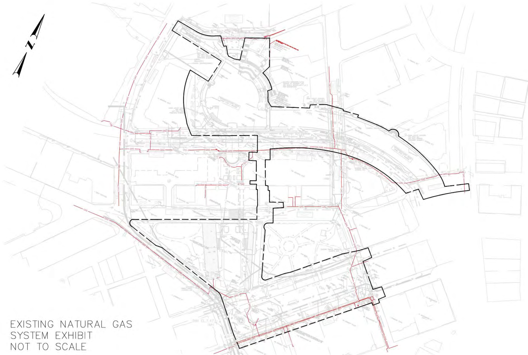
Figure 14 - Existing Natural Gas System
