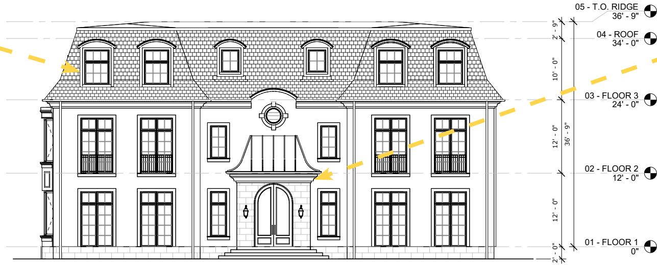
③ EAST ELEVATION - PROSPECT STREET 1/8" = 1'-0"
