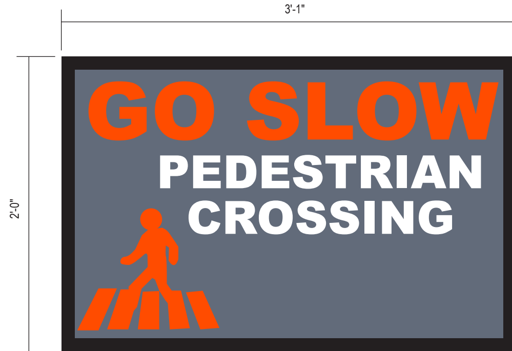
A Sign Elevation - Front View Scale: 1 1/2"=1'-0"
