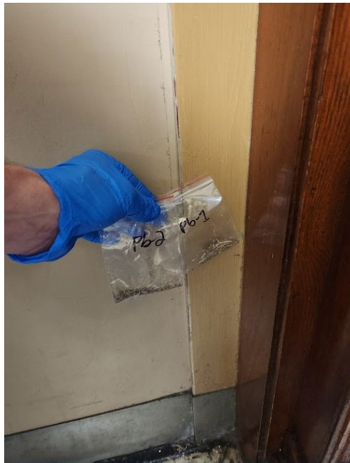
Positive LBP samples from elevator entry panels and trim.
