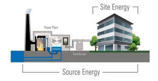
To be able to compare buildings of different sizes, the source energy or the site energy are divided by a building's square footage to determine the energy use intensity.
